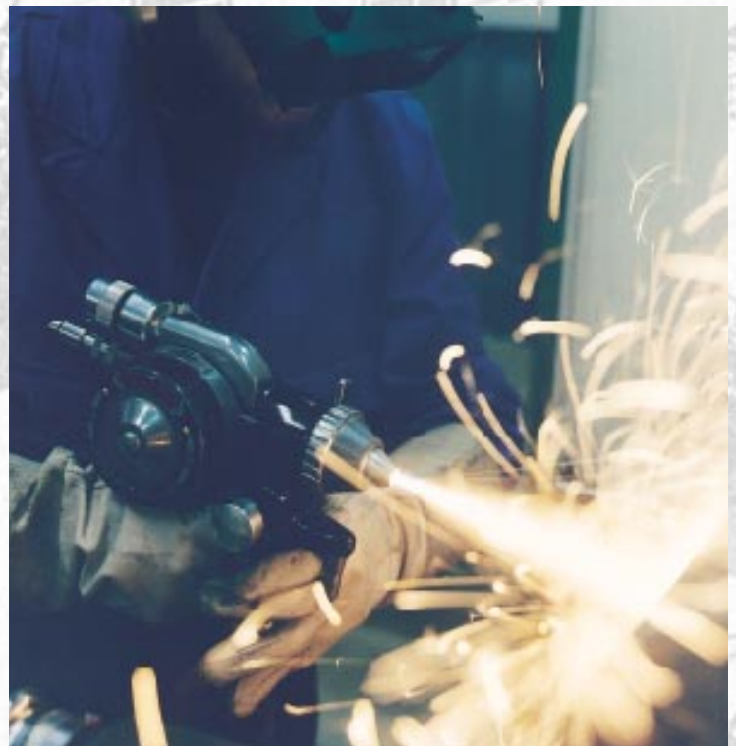
Wire flame spraying for the investigation of coating materials with melting points of 400 °C to 2600 °C
