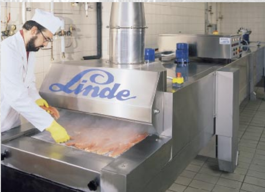
Type L freezing tunnel developed by Linde for the quick-freezing of e.g. meat, fish, breads, pastries, vegetables and fruits. Fast, product-adapted removal of heat guarantees food quality and a high throughput rate.
