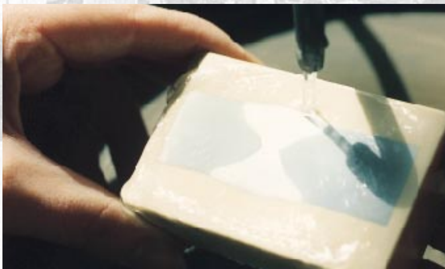
Macro sections of weld specimens being prepared in the laboratory for wet chemical and metallographic analysis to display and inspect the optimal penetration.
