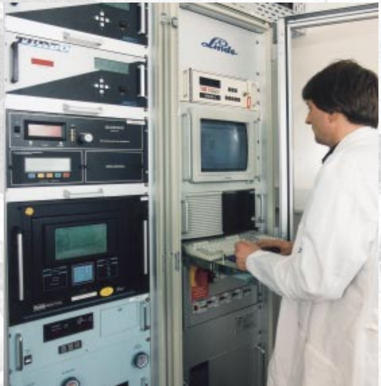
Test run of a monitoring system for the ppb range with automatic calibration
