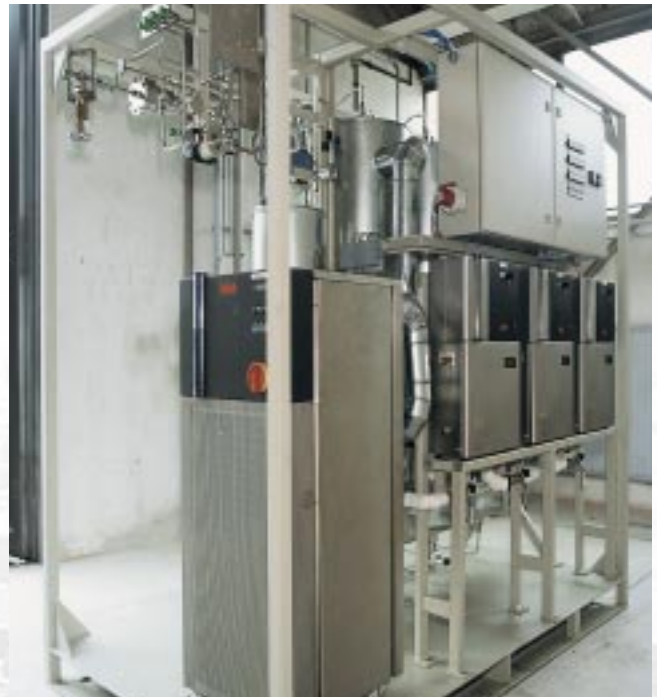
Pilot plant for the optimisation of gas purity in the Specialty Gases Laboratory
