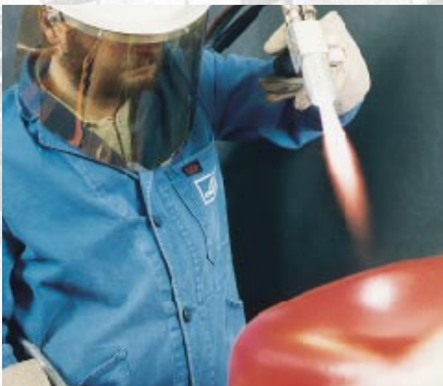
Thermal processing of plastic with an oxyacetylene flame. Specially designed spraying systems allow even very low-melting plastics to be worked on with this flame.
