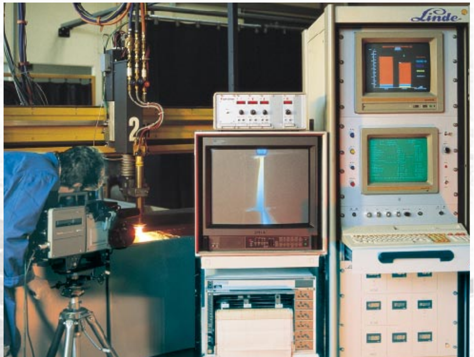
Oxyfuel gas cutting (top) and plasma-arc cutting (bottom) are studied under plant conditions with modern CNC cutting machines.
