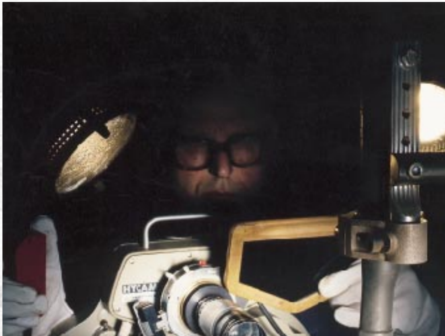
A high-speed camera filming the GMAW process at 10,000 frames per second. Metal transfer during welding can be seen in detail when the film is viewed in slow motion.
