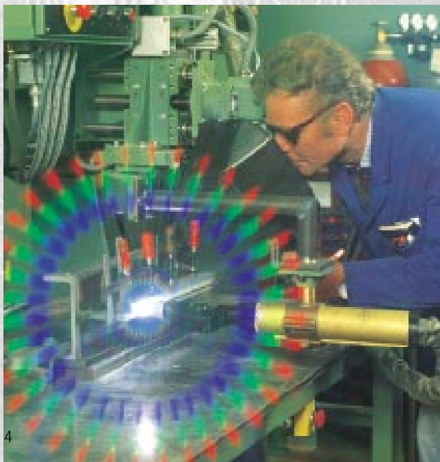
Experimental robot turntable system with 8 independently programmable axes with which overall welding concepts as well as part and torch tolerances are worked out for customers on parts supplied by them
