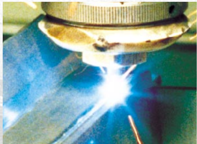
Laser-beam welding with LASPUR®-grade helium (field magnet of an electric motor)
