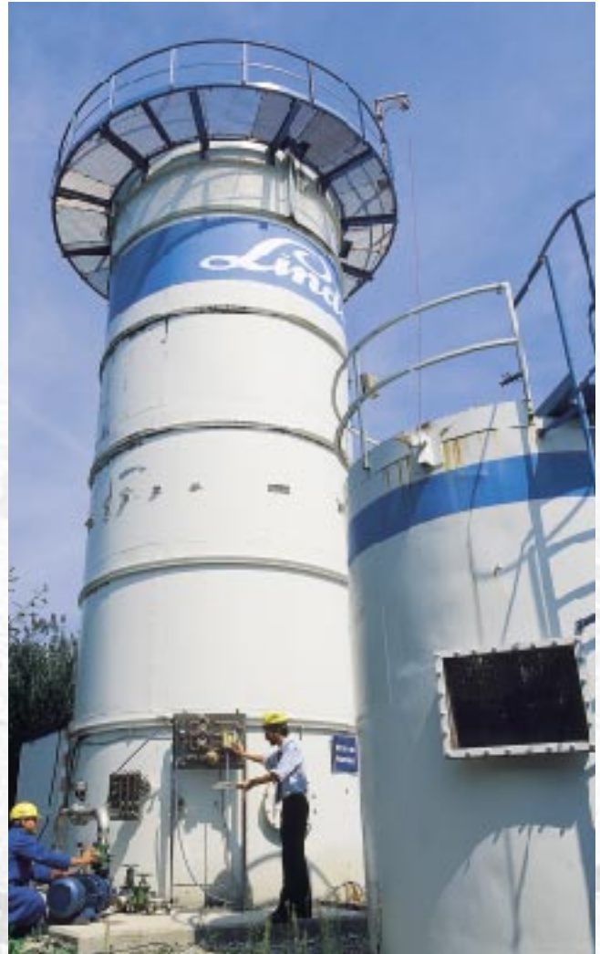
Water tower used to determine the oxygen transfer capacity of various injection systems
