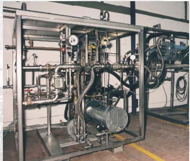
Experimental and demonstration machine for recovery of valuable substances or contaminants from gas streams (cryogenic condensation with liquid nitrogen).
