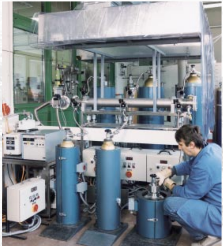
Evacuation with a turbo-molecular pump within the frame of cylinder pretreatment
