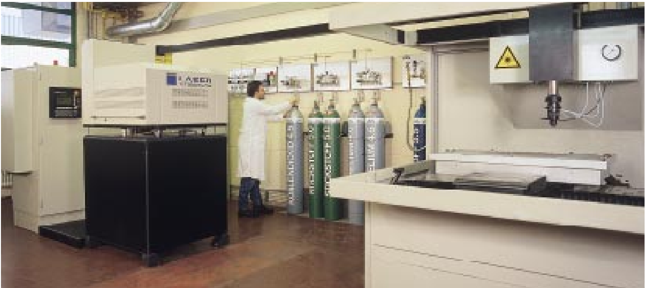
CO 2 laser cutting machine used to obtain empirical values for flexible, economical fabrication. Linde has exactly the right LASPUR® working gas for every requirement, be it cutting, welding or surface treatment.
